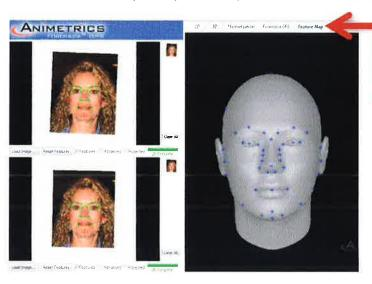
Click the **Feature Map** tab to display a model with the correct feature point placement. When you click one of the crosshairs on the probe image, the crosshair on the Feature Map model will be highlighted in green to show you the proper placement.
